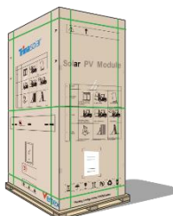
Vertical portrait package (long-side vertically placed)
